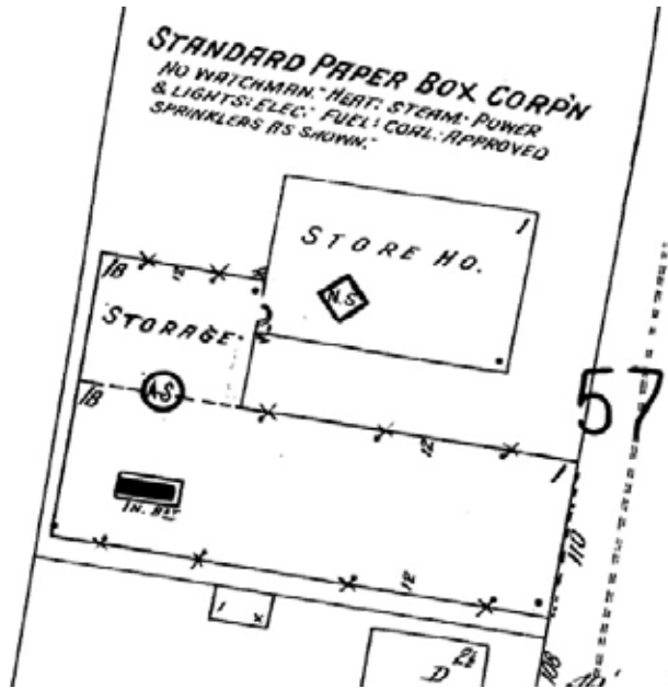
Figure 2 Detail from 1923 Sanborn Fire Insurance Map showing single-story, L-plan Main Building (Building 1, 1914) and frame Store House (Building 2, ca. 1920)
